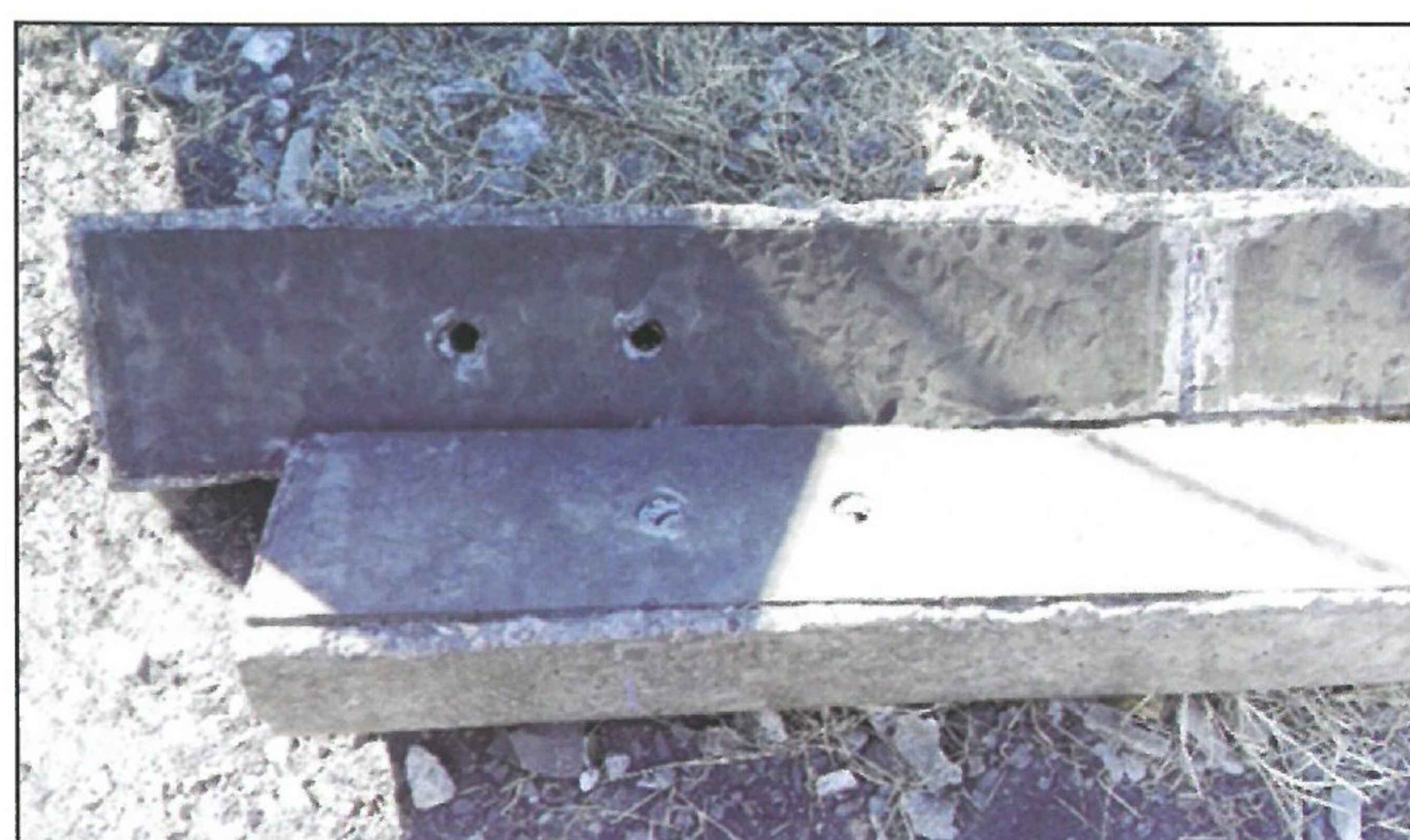
Fig. 15: Removed padded sleepers after more than 1 billion load tons of traffic – no signs of damage
